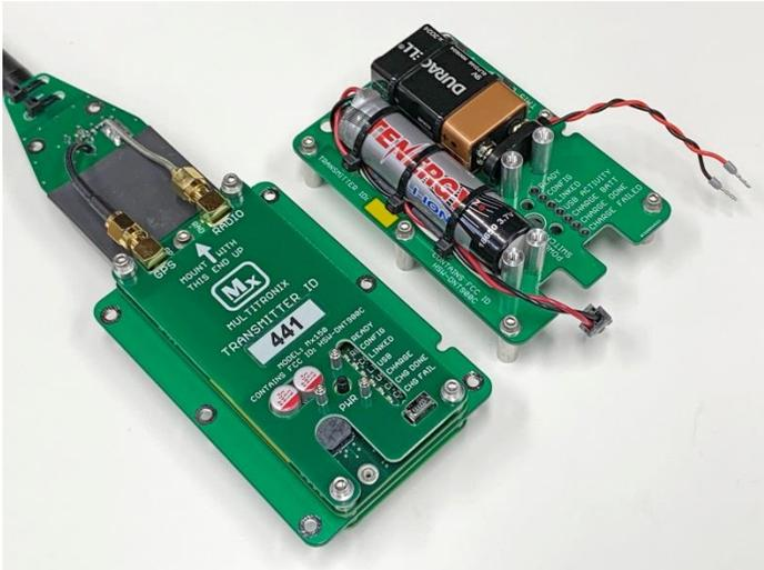
This picture shows the Mx230 Option-20 transmitter configuration with the Option-25 battery board alongside it. The battery board is now ready to be mounted over the top of the transmitter.
