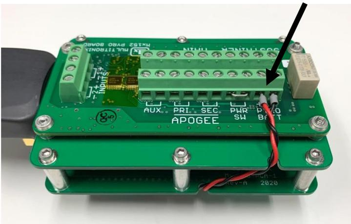
**Step 10:** The battery board is now properly mounted to the transmitter. The last step is to connect the pyro battery leads to the PYRO BATT terminals on the pyro board. **Be extra careful to get the polarity right!** Also while hooking them up, make sure the battery leads do not touch each other or any exposed metal on the pyro board.
