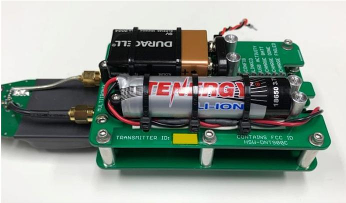
**Step 7:** Lay the battery board all the way down onto the top of the transmitter. It should now be resting on the six metal standoffs.
