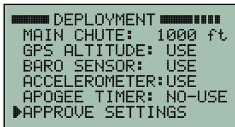
You can also select **MAIN DEPLOY** and then change the number from 1000 feet to be something else if you need to use a different altitude for deploying the main parachute.
