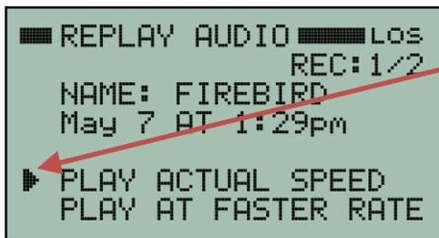
To start playback, point the cursor to either line labeled **PLAY** and then press the right arrow button. There are two options for playback. One plays the audio at the actual speed it was recorded. The other option plays it at a faster rate by eliminating long periods of silence between sentences.
