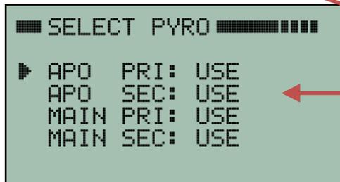
To specify which deployment channels are being used, select **SPECIFY USE**.
