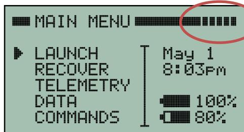
A signal strength indicator is shown on every screen. Maximum signal strength is “five bars” as is shown here.
