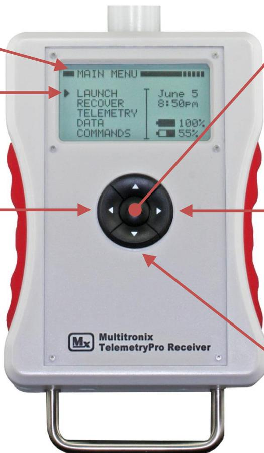
Center button works just like the “enter” key on a computer keyboard. It is used to enter data and commands. It also serves as the power switch.
