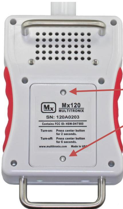
Loosen two screws to remove battery compartment door.
