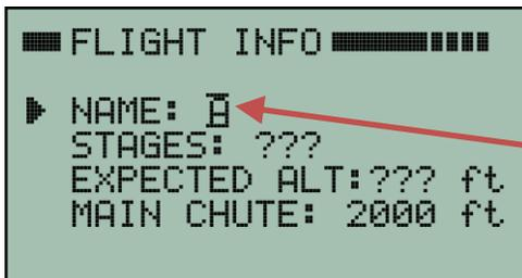
Position the cursor so that it is pointing to **NAME** and press the right arrow button to enter edit mode. The three question marks will disappear and the letter "A" will appear with edit bars blinking above and below it. Use the up and down buttons to change the letter as needed. Pressing and holding an up or down button will automatically scroll through the available letters and numbers.
