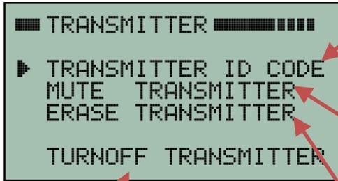
Click here to bring up a screen that allows you to set the transmitter ID code in the receiver. The receiver must be set to the same ID code as the transmitter in order to establish a radio link. See section 5 on page 8 for more details.
