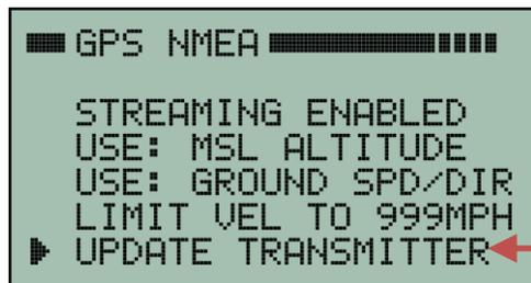
When you change one or more settings, a new line will appear at the bottom of the screen. It is blinking and says UPDATE TRANSMITTER. Position the cursor on the UPDATE TRANSMITTER line and press the center button to send the new settings to the transmitter. The new settings will take effect immediately. They are also permanently saved in the transmitter even if it is power cycled.
