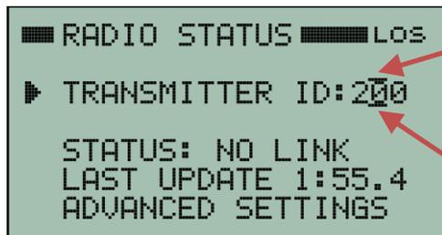
Edit bars will now be blinking above and below a digit in the ID code number. They indicate which digit will be changed by pressing the up or down arrow buttons. The edit bars can be moved right or left by pressing the right or left arrow buttons. This scheme allows you to set each digit in the number.
