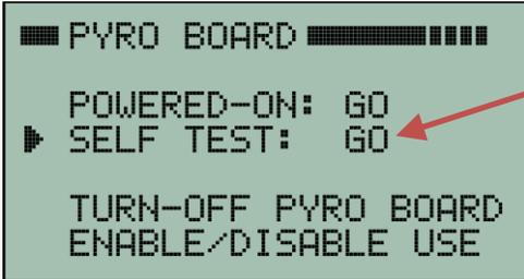
When the pyro board is powered-on, it performs an internal self-test to make sure there are no detectable hardware failures. If self-test passes then it will be a GO as is shown here. If self-test fails, then position the cursor pointing to **SELF TEST** and press the right arrow button to see why it failed.
