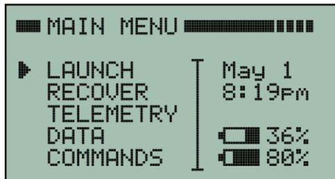
To setup the pyro system, go to the MAIN MENU and position the cursor at **LAUNCH**, as shown here. Then press the right arrow button to see the LAUNCH STATUS screen.
