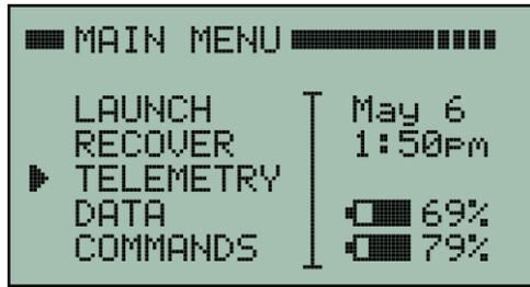
It is recommended to switch to the TELEMETRY screen just prior to launch so that it will be easy to see the real time telemetry data during the flight. This is done by returning to the MAIN MENU and positioning the cursor so that it is pointing at **TELEMETRY**. Then press the right arrow button or the center button.
