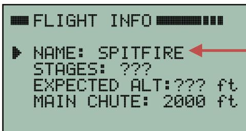
Finish out the rest of the name and then press the center button to enter it. This will exit edit mode and allow the buttons to resume normal operation.
