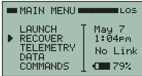
Go to the MAIN MENU and move the cursor so that it points to **RECOVER**. Then press the right arrow button to enter recovery locator mode.
