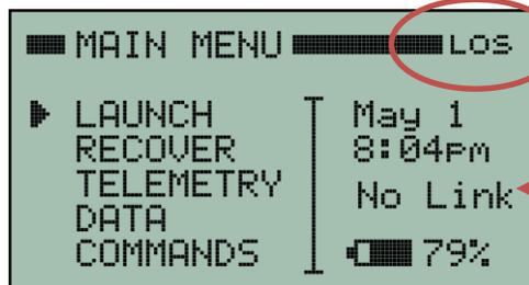
The signal strength indicator will blink “LOS” indicating “Loss of Signal” when the link with the transmitter has been completely lost or has not yet been established.
