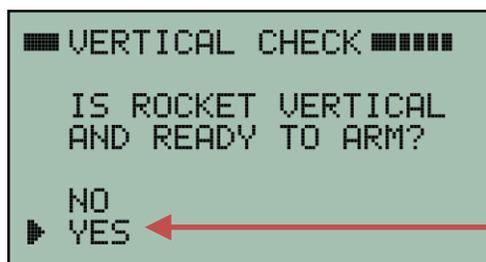
Before the system will arm itself it requires that you confirm the rocket is vertical. This makes sure the proper accelerometer orientation has been established.
