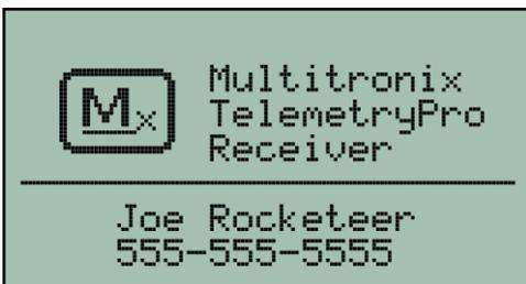
This shows how the owner's name and phone number are displayed on the first screen after power-on.
