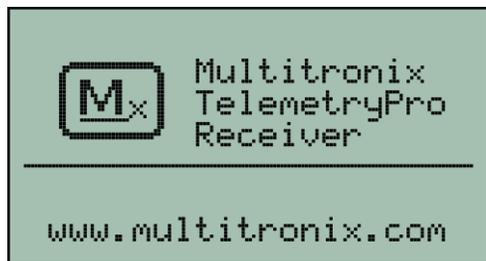
This screen will be shown when the receiver is first turned on. Press any button to proceed to the main menu.
