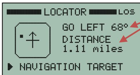
Bearing and distance to the rocket will change as you walk around with the receiver. The receiver must be held with the antenna pointing in the direction you are walking in order for the bearing to be valid. In other words, the arrow on the “radar screen” must be pointing in the direction of travel. The distance to the rocket is always valid even while you are stationary.
