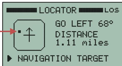
The “radar blip” is solid when a valid measurement is being displayed. This occurs when the receiver is moving at least at walking speed. The “radar blip” will blink when it is displaying the last valid measurement but that measurement is more than 10 seconds old.
