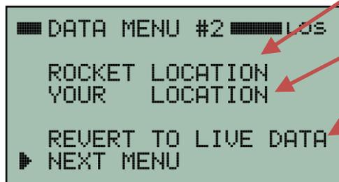
View the most recent GPS coordinates and altitude (AGL) received from the transmitter in the rocket.
