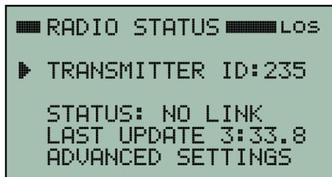
Once all the digits have been properly set, press the center button to enter the transmitter ID code number. This will also exit the edit mode and allow the buttons to resume normal operation. In this example, the ID code has been set to 235. The ID code stays set even if the receiver is powered-off. It does not need to be set every time. Only if it needs to be changed.
