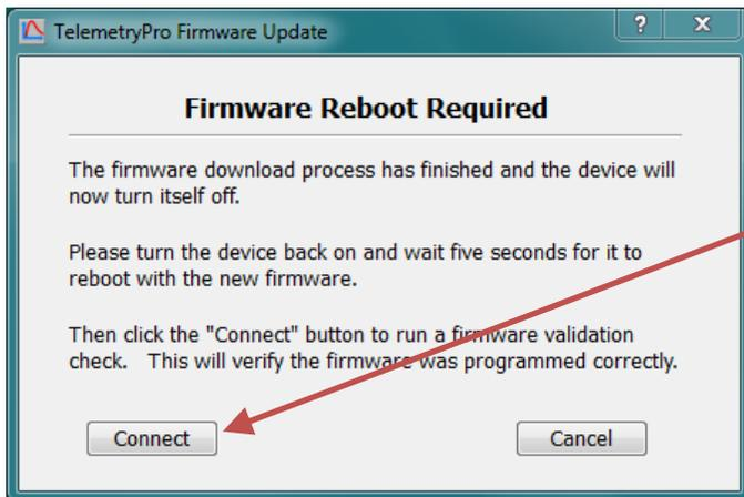
When this “Firmware Reboot Required” window appears you just need to power-on the device, wait at least five seconds and then press the **Connect** button. This will start a validation check of the new firmware to verify it was programmed correctly.
