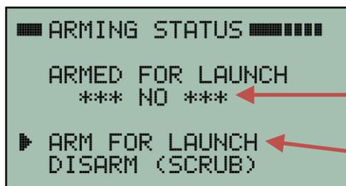
The system is not yet armed for launch as indicated by a blinking "NO".
