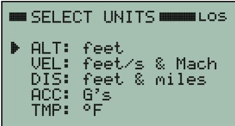
To change a selection, just move the cursor to the desired parameter and press the right arrow button to cycle through all the available options.
