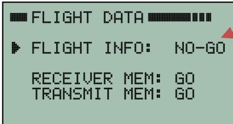
Next we turn our attention to the FLIGHT INFO since it indicates NO-GO. Position the cursor onto this line and press the right arrow button to view the flight plan screen.
