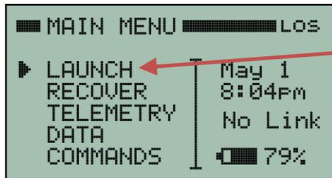
Go to the MAIN MENU and position the cursor with the up/down buttons until it is pointing to **LAUNCH** as is shown here. Then press the right arrow button to see a launch status menu.
