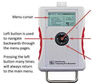
Press and hold the center button to turn the receiver on or off.
