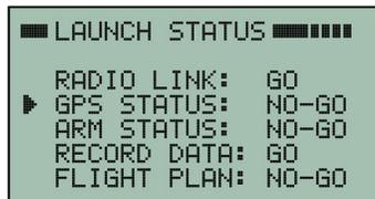
The LAUNCH STATUS screen shows all the go/no-go criteria. If any are no-go then position the cursor onto the line that is no-go and press the right arrow button to enter a menu or status screen for that item. The receiver will prompt you for any info it needs.
