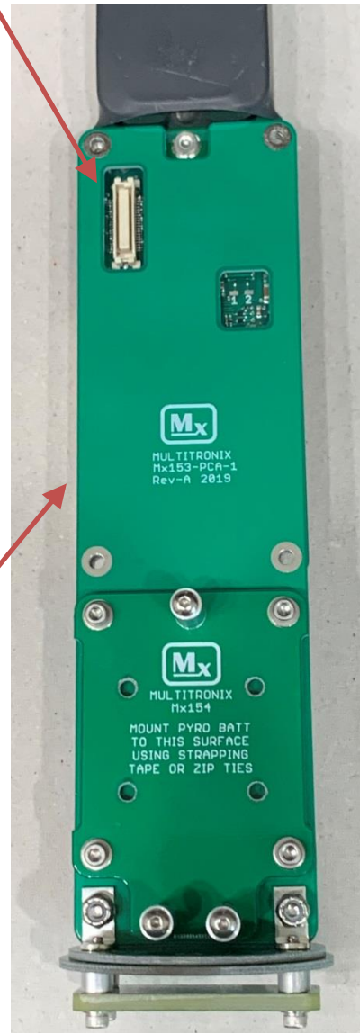
Battery board placed over the back side of the transmitter.
