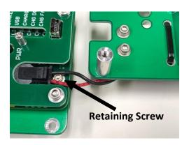
**Step 7:** Spread the red and black battery leads apart and remove the small retaining screw. It requires a 5/64" hex driver.
