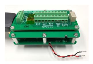
**Step 1:** Lay the unit on a flat surface with the pyro board facing up. Disconnect the red and black pyro battery leads. Be careful not to allow the ends of the leads to touch each other or any other metal on the pyro board.
