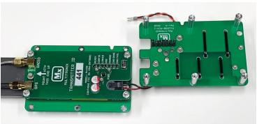
**Step 6:** Lay the battery board down on the surface so that it is end to end with the transmitter. The system battery leads are still connected so they will limit the final position.
