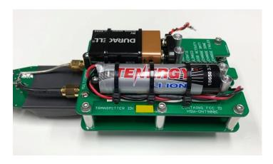
**Step 3:** Hold everything together and carefully flip the unit over so that the battery board is now facing up as shown here.
