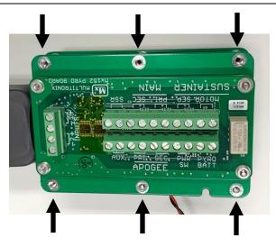
**Step 2:** Remove six socket head screws from the locations indicated above. They require a 3/32" hex driver or Allen wrench.
