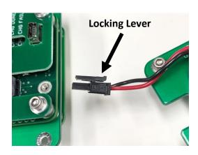
**Step 8:** Press down on the locking lever and pull the battery connector straight out and away from the board.
