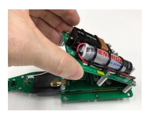
**Step 4:** Lift up on the forward end of the battery board and rotate it about the aft end.
