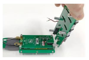
**Step 5:** Continue rotating the battery board upside down onto its topside.
