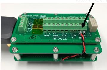
**Step 10:** The battery board is now properly mounted to the transmitter. The last step is to connect the pyro battery leads to the PYRO BATT terminals on the pyro board. **Be extra careful to get the polarity right!** Also while hooking them up, make sure the battery leads do not touch each other or any exposed metal on the pyro board.
