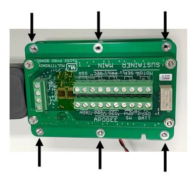
**Step 8:** Hold everything together and carefully flip the unit over so that it is now resting on the battery board. The pyro board should now be facing up as shown here.
