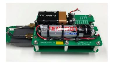
**Step 7:** Lay the battery board all the way down onto the top of the transmitter. It should now be resting on the six metal standoffs.
