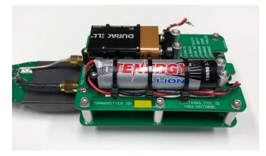
**Step 3:** Hold everything together and carefully flip the unit over so that the battery board is now facing up as shown here.
