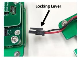
Step 8: Press down on the locking lever and pull the battery connector straight out and away from the board.
