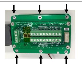
**Step 2:** Remove six socket head screws from the locations indicated above. They require a 3/32" hex driver or Allen wrench.
