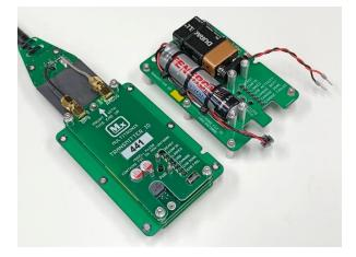
The battery board should now be completely disconnected as shown here.
